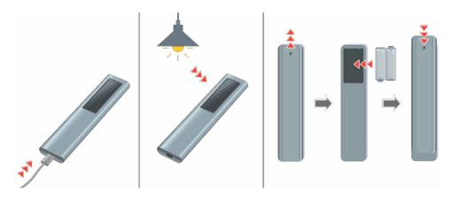
If you cannot see infrared signals, charge the remote control by using the USB port (C-type) on the bottom, or turn over the remote to expose the solar cell. If the remote control has batteries, replace them with new ones.
