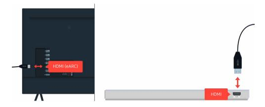
If no sound comes out of your Sound Bar, and if it is connected to the TV with an HDMI cable, check the HDMI (eARC) connector on the back of the TV.
