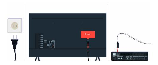
If the remote control sensor is not turned on, unplug the power cable and plug it back in.
